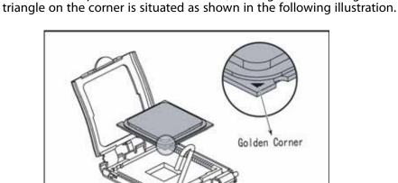
**9** When the processor is oriented correctly and in place, press it firmly into the socket, rotate the load plate into place, and push down the load lever until it clicks into place.
